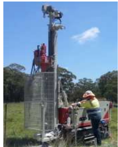
Geotechnical investigations use a small drill rig towed on a trailer
