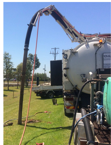
NDD uses a vehicle about the size of a council rubbish truck
